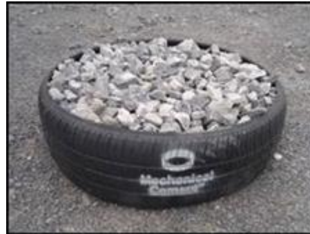
FIGURE 2 MECHANICAL CEMENT® GEOCYLINDER STONE FILLED TDGC
